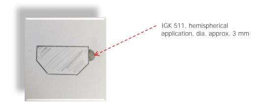
The position of the IGK 511 "round string" must be centrally on the side. After pressing, IGK 511 may neither enter the gap between the discs nor the bevel of the spacer.
