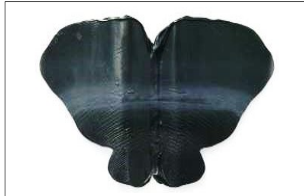
Figure 7: Unfold the foil - Negative test = inadequate mixing
