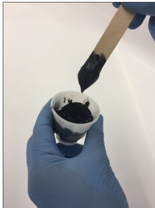
Figure 9: Material shows rubber-like behavior: snap time reached
