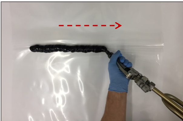
Figure 4: Apply the bead in the fold direction
