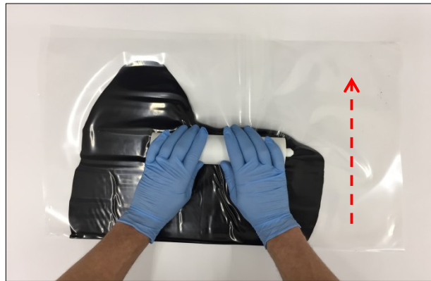
Figure 7: Press the bead only in direction perpendicular to fold
