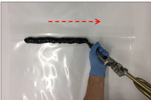
Figure 6: Apply the bead in the fold direction
