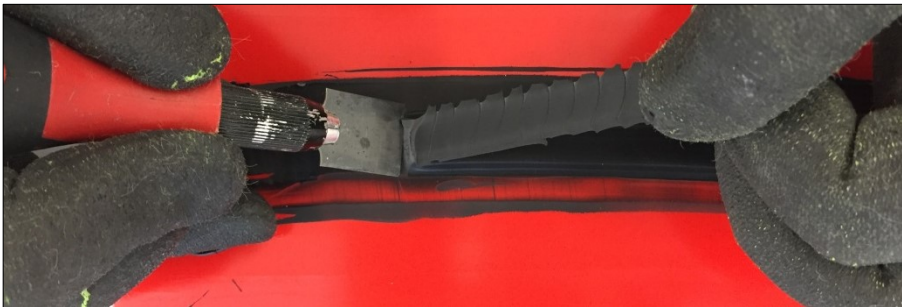
Figure 19: Peel adhesion test on enameled glass: cutting the bead while pulling
