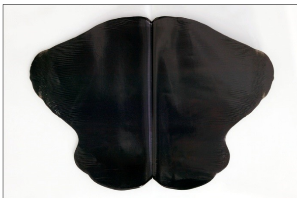
Figure 8: Unfold the foil - Positive test = ideal mixing
