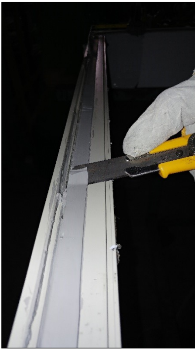
Figure 29: Testing joint adhesion along the whole frame – Good adhesion.
