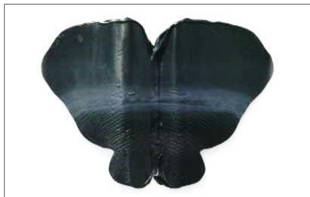
Figure 9: Unfold the foil - Negative test = inadequate mixing
