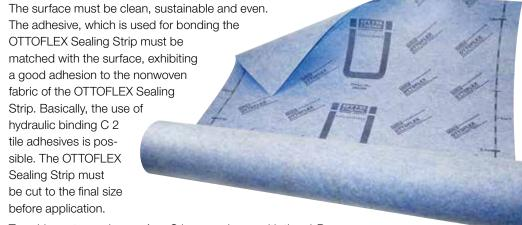
To achieve stress classes A or C in accordance with the abP as well as A0 in accordance with the ZDB, the sealing strip in the joint area must be bonded with at least 5 cm of overlap using OTTOCOLL® M 500.
