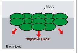
**The improved protection against mildew** is of particular relevance to joints that require maintenance. Despite the improved protection against mildew, however, these should still be regularly inspected and replaced if necessary.
