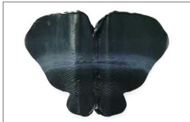
Figure 7: Unfold the foil - Negative test = inadequate mixing
