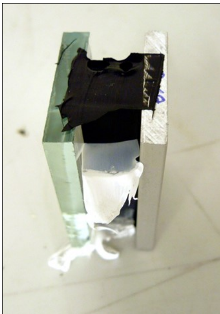
Figure 19: Remove spacers after 1 day, remove e-PTFE tape after 7 days (1-part adhesives).
