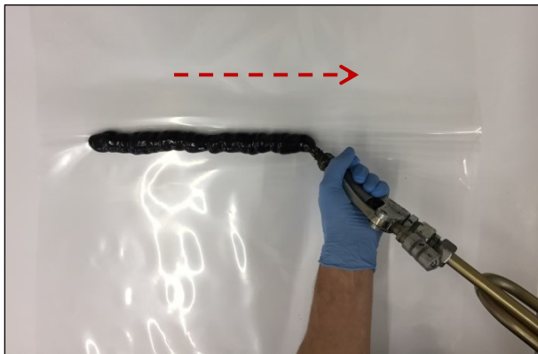
Figure 4: Apply the bead in the fold direction
