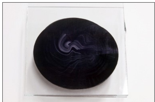
Figure 3: Negative test = inadequate mixing
