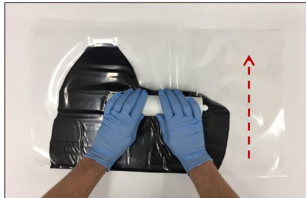
Figure 5: Press the bead only in direction perpendicular to fold
