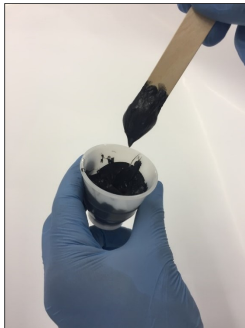
Figure 9: Material shows rubber-like behavior: snap time reached
