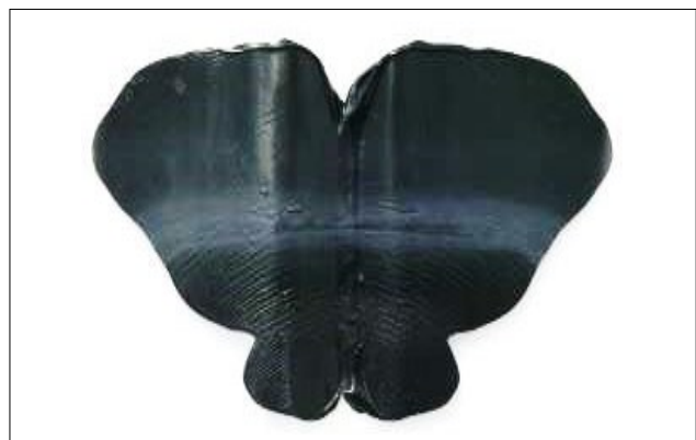
Figure 9: Unfold the foil - Negative test = inadequate mixing
