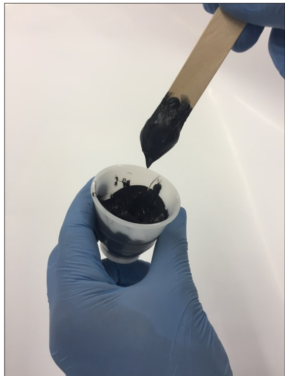
Figure 12: Material shows rubber-like behavior: snap time reached
