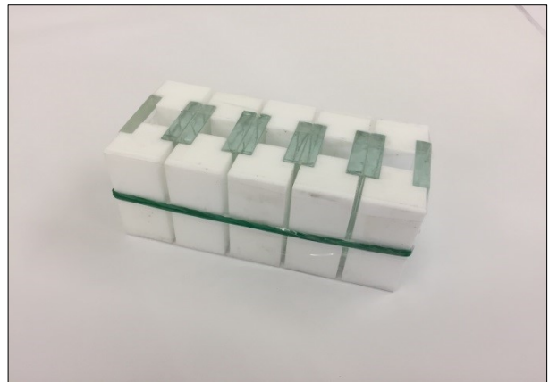
Figure 21: Arrangement and fixation of the samples with a rubber band and tape
