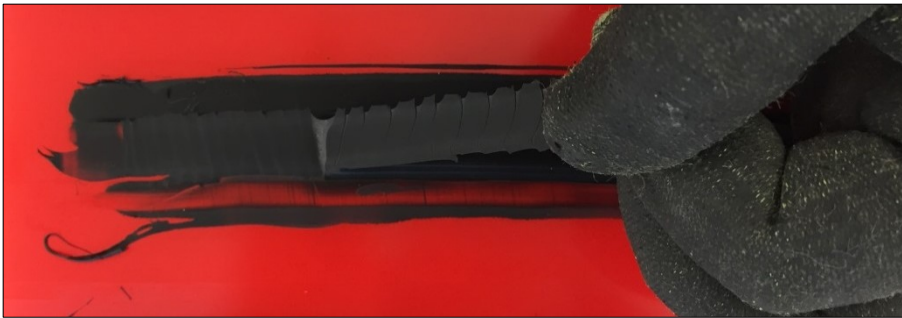
Figure 18: Peel adhesion test: pulling the bead apart, 100% cohesive failure occurring
