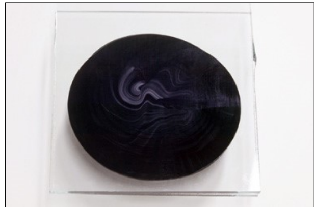
Figure 5: Negative test = inadequate mixing
