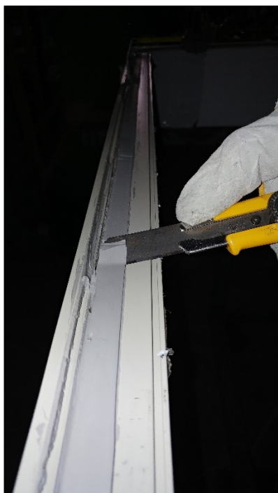
Figure 29: Testing joint adhesion along the whole frame – Good adhesion.
