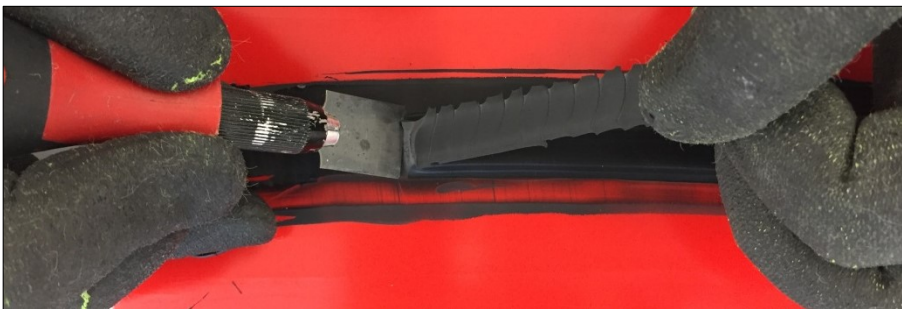
Figure 19: Peel adhesion test on enameled glass: cutting the bead while pulling
