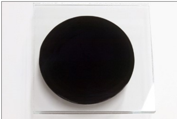
Figure 4: Positive test = ideal mixing
