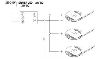
For LED STRIP applications which are longer than 5 m, it is recommended to use multiple power supplies to reduce the effects of natural voltage drops. Applications with multiple branch circuits are possible with suitably sized DRIVERS.
